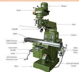
The **vertical milling machine** is a precision tool used for shaping and fabrication by the removal of stock typically from metallic work pieces
