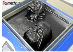
where a sheet of plastic is heated to a forming temperature, stretched onto a single-surface mold, and forced against the mold by a vacuum. This process can be used to form plastic into permanent objects
