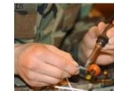
Soldering is a process in which two or more items are joined together by melting and putting a filler metal into the joint,
