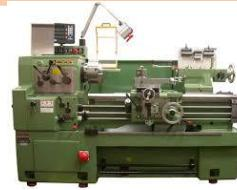
The **Centre Lathe** is used to manufacture cylindrical shapes from a range of materials including; steels and plastics.
